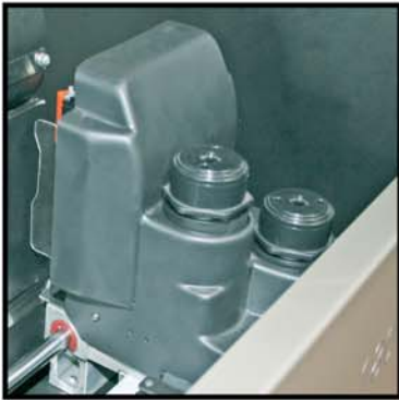
Dual Ink Tanks on Printhead Carriage
